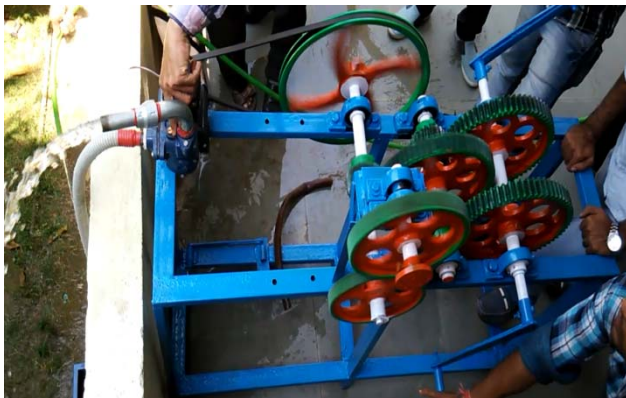
Fig. 3.3 Human handle powered irrigation system.
