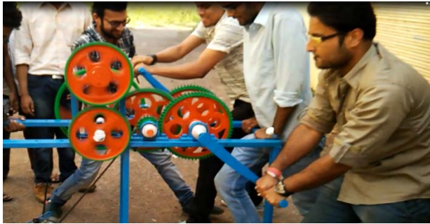
Fig. 3.2 Human handle powered mechanical system for electricity generation.
