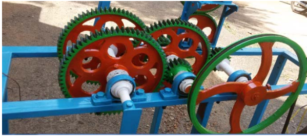
Fig. 2.1: Human muscle powered Speed increaser.
